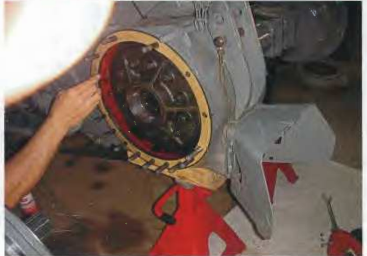
After greasing the paper seal it was fitted to the bolts.
